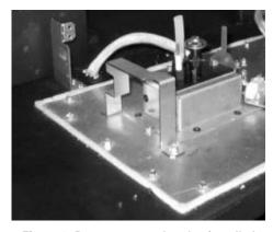
Figure 6: Burner support bracket installed
