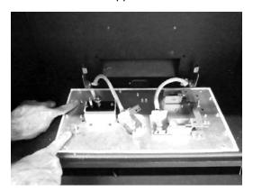
Figure 5: Burner support bracket screws location
