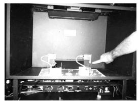
Figure 1: Accent light bracket screws location
