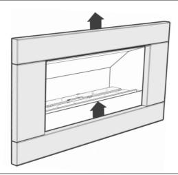
Now slide the fascia towards you until it falls into the additional slot, unplug the electrical cord. Now you can rest the Fascia on the ground.
