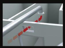
When placing outlets in rooms other than the room the appliance is installed, it is important to allow for back flow to equalise pressure between the rooms, and to allow for temperature regulation.
