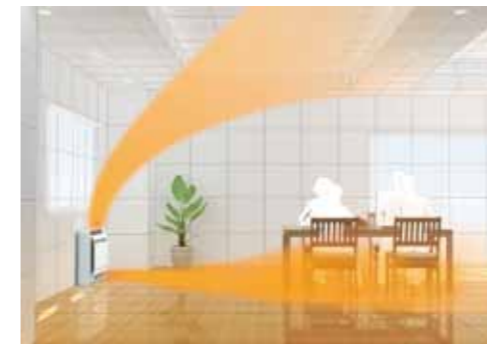
Double airflow keeps the floor warm during heating operation.
