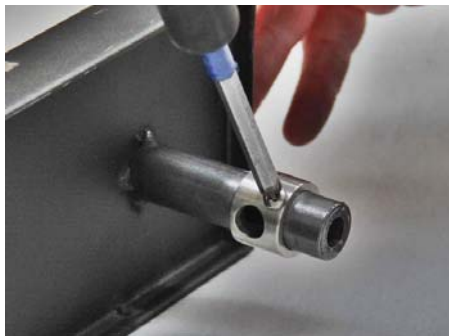
ULPG/Propane 11mm hole exposed
