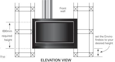
\* Note: Standard Fascia finishes flush with the bottom of the firebox so ensure a neat finish to plaster/gyprock.
