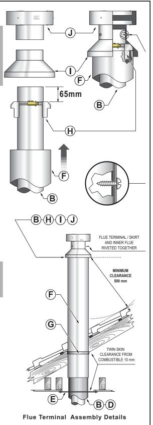
Flash roof penetration by approved methods. (Roof flashing materials are not included in flue kit).
