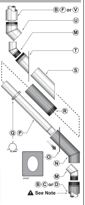
The vertical length of flue pipe between the heater and the first inner 45° elbow (M) (FLFTWKIT) should be as long as the installation allows, and at least 900mm.
