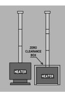
Direct rigid flueing is used when running a flue direct from appliance to the termination point. The flue components supplied in Rinnai FLFKIT05 are best suited for this type of installation.
