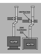
When an obstruction prevents the use of a direct rigid flue run from the appliance to the termination point a FLFBEND kit consisting of two 45° offsets can be used to divert the flue.
