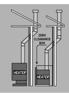
Through wall rigid flueing is used to divert a flue run from appliance through an exterior wall to the termination point.
