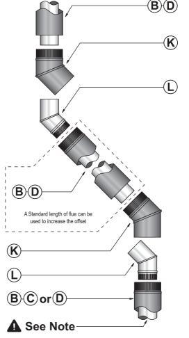
At this point to extend the offset length use a combination of standard inner (B) and outer (D) flue pipe lengths, joining the inner flue sections with three galvanised screws or rivets.
