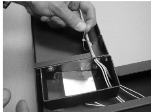
Figure 6: Securing the lock-tie
