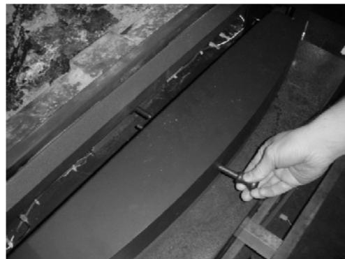
Figure 22: Tightening the air control rod
