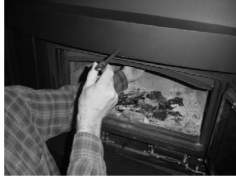
Figure 24: Attaching the extension rod
