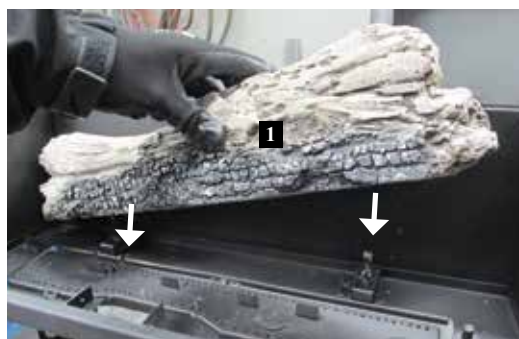
Logs 1 - fits over pins behind burner
