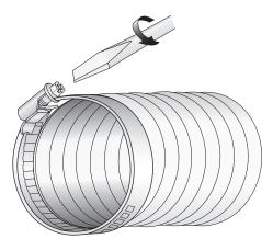
Using a flat head screwdriver, unscrew the flue clamp as necessary until it fits over the end of each of the flexi flue pipes.
