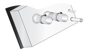
Stretch out the end of each flexible flue pipe to ensure the flue clamps grip tightly. Slide the two flexi flue pipes over the corresponding pipes at the rear of the firebox.
