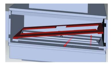
11) Remove left and right screws from the burner legs.
