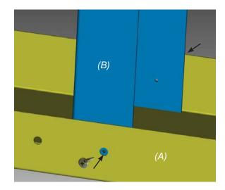
4) With all 4 - (B) pieces secured to the bottom with 2 screws (1 on each side) (A) can be placed into position, as shown below. Ensure all tabs on the (A) are bent to 90° and oriented to each (B) as shown in step 2.
