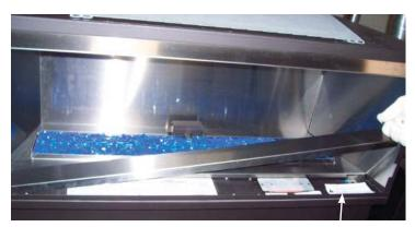
**10)** Remove the burner tray by lifting up and out.
