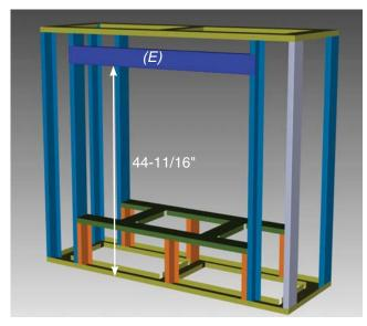
12) Line up screw holes on (E) (header) and (B) (inner vertical support). Secure with 2 wafer screws on each side (4 total) as shown below. This will now be the front of the frame.
