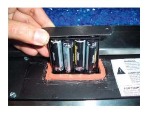
3) Install 4 - AA batteries and reverse steps.
