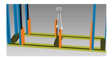
Position (D) on top of (C) pieces - line up screw holes and secure (D) to (C) with 12 wafer screws.
