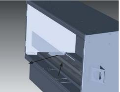
6) Remove the screw and panel clip on the right side. Remove the right side panel once the clip has been removed.
