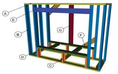
1) Place top/bottom (A) on the ground - flat side down. Bend the tabs up to a 90° angle.
