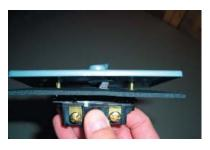
6) Mount completed switch assembly with cover plate to the electrical box using 2 outer holes on cover plate. (Shown without facing material)
