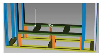
Measure 44-11/16" from floor (bottom of the header location) line up (E) (header) with appropriate screw holes.
