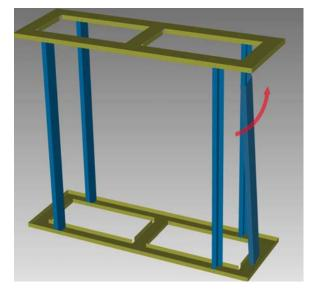
7) Llne up screw holes on top / bottom (A) with each (B)- secure with 3 wafer screws each on top and bottom - 6 screws in total for each outer (B) (3 top- 3 bottom).
