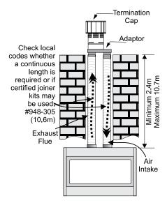
Note: When installing the flueing, identify the flues.
