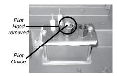
**10)** Remove the pilot orifice with the allen key.
