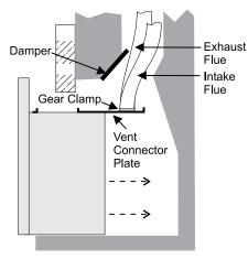
Be careful not to damage thermal insulation when sliding on vent connector plate. This could cause blockage.
