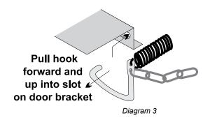
To remove the flush door, reverse the above steps.
