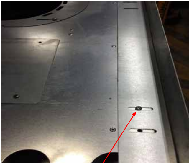
Nailing strip installed with slotted side on unit. The slot allows the movement of the nailing strip to be adjusted depending upon thickness of finish material.
