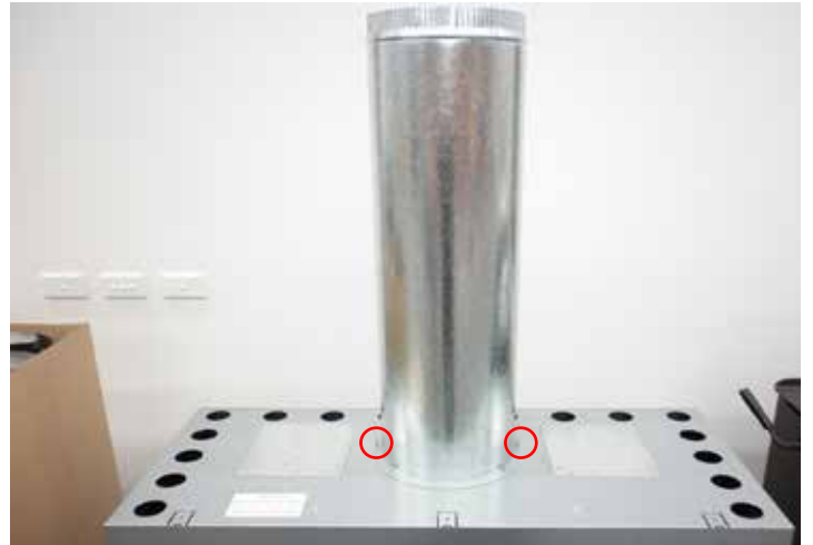
5. Bend up the 2 tabs on each side of the 10" flue and secure via self drilling screws
