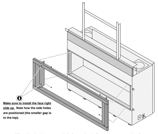
When tightening the screws, push the face against the facing to ensure a seamless fit.
