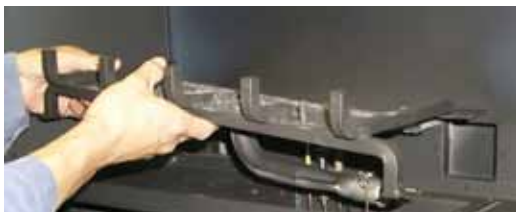
Remove the left and right screws and then lift out the burner/grate assembly.
