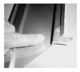
8 Slide the adjoining side trim onto the "L" brackets and spacers. Repeat steps 6-8 for the opposite side. **NOTE**: If the "L" brackets are too tight, loosen a few turns. Do not tighten the "L" brackets at this time.
