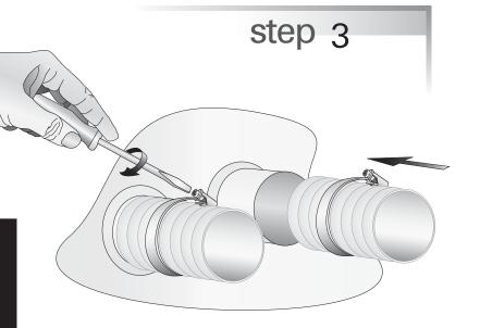
Tighten flue clamps to secure flues to the firebox.
