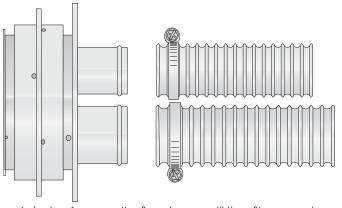
As in step 1, unsrew the flue clamps until they fit over each of the flue pipes. Slide the two flues over the corresponding pipes on the base of the cowl.
