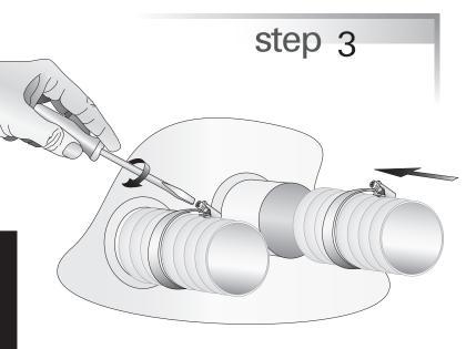
Tighten flue clamps to secure flues to the firebox.
