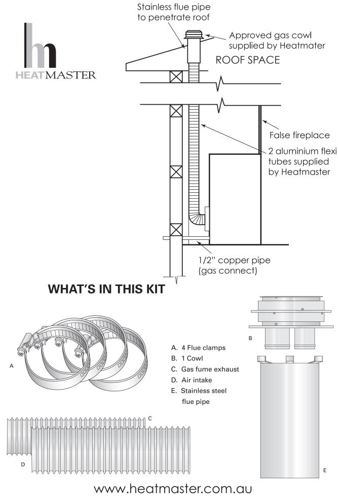
Flue installation should be read in conjunction with Enviro quick step installation manual.
