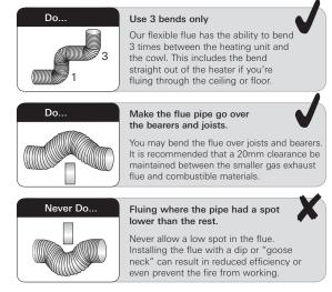
N.B. Remember not to have a dip anywhere in the flue It is recommended that 20mm clearance is maintained between the smaller extraction flue and combustible material
