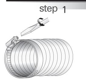
Using a flat head screwdriver, unscrew the flue clamp as necessary until it fits over the end of each of the flexi flue pipes.
