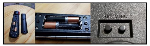
The menu itself is easy to use, and allows for you to toggle the Temp setting from F to C (the default is F), adjust the display brightness, set the decimal point (so it doesn't read in whole numbers), and finally adjust the amount of time before the unit enters "sleep mode".
