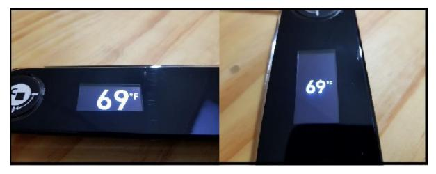
The Snap Check also has an inbuilt "accelerometer" allowing the screen to rotate when the thermometer is moved at various angles, making reading easy whatever way it's held.
