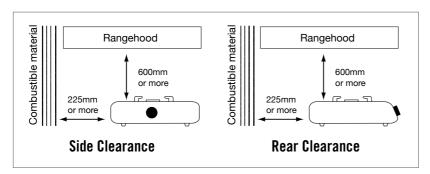
The minimum clearance from the appliance to the rear or sides of all combustible surfaces must be no less than 225mm. When the appliance is installed abutting a side or rear surface the surface must be made of non-combustible materials such as ceramic tiles or glass splash backs. If the surrounding surfaces are constructed with a combustible material, contact your local Gas Authority for information on clearances required.
